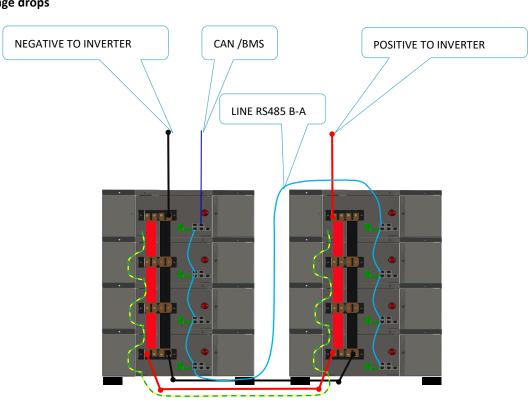
After all cables and bar buses have been connected and the inverter has been set correctly, place the rocker switches (see section 5.4) of all batteries on ON (I). Try to start the system by turning on only the master module: if the installation is set correctly all modules will turn on in sequence.
