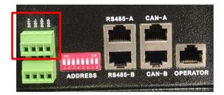
Using the PC software, you can define dry contact activation thresholds based on the % SoC value of the battery. After connecting to the battery with the software using the installer password, simply go to the DO Setting page.
