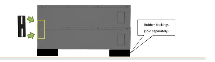
Step 4: Once each battery has been installed horizontally, the feet supplied with the battery in standard configuration can be removed and installed through the modules to constrain the modules on both sides.
