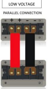
The low voltage screw terminal only supports parallel connection with maximum voltage 60V CAUTION> Connecting these terminals in series will cause serious damage to the battery
