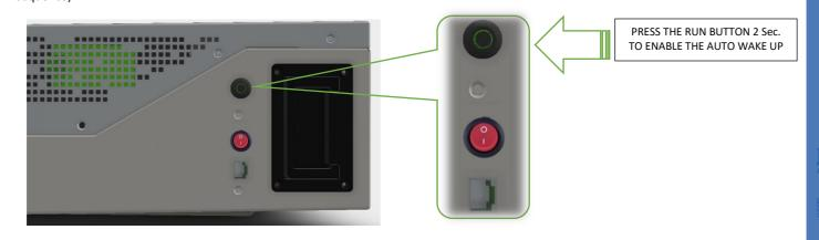
It is essential to check the startup progression and make sure that all LEDs of the RUN BUTTON are ON and showing steady GREEN lights after the wake-up process (the entire process might take up to 30-45 seconds in case of 15 batteries).
