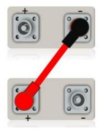
Fast Connector terminals only support series connections up to 1000Vdc CAUTION> Connecting these terminals in parallel will cause serious damage to the battery
