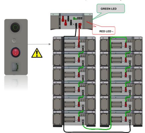
**Information:** Arrange the cables according to the specific installation requirements, always paying attention to minimize the length of the cables to avoid voltage drops.
